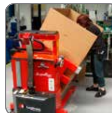
Optimum working conditions: The user can reach the contents without stretching and straining the back.
