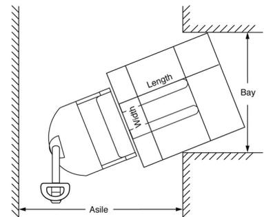
Aisle dimensions listed above assume 4" between loads. Use the larger dimension; load width or load length. For ease of use and add 6" to 12" for operator clearance to the appropriate specifications listed above. Truck performance may vary due to application requirements' and changes in model design.
